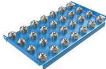
BPD DROP IN CONVEYOR FRAME STYLE BPD is designed to replace rollers in existing sections of gravity roller conveyor and is typically used as a transition/positioning area.
