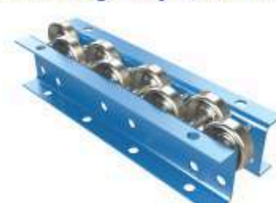
WRB - HEAVY DUTY PALLET RAIL WRB's opposing channels offer a sturdy configuration to cover longer spans, while the staggered wheel pattern conveys irregularly shaped loads.
