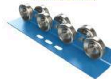
WRK - LIGHT DUTY RAIL FOR TOTES, BOXES, CARTONS WRK's staggered wheel pattern conveys irregularly shaped loads. The angle frames are also ideal for floor mounted applications.
